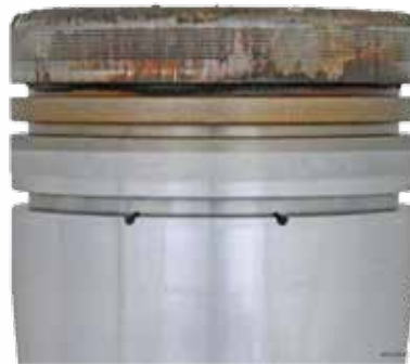
Pistons accumulated very low deposits (thrust side down)
