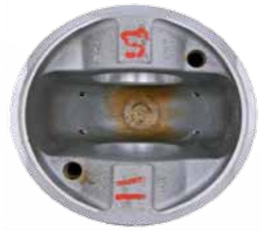
Clean undercrowns facilitated oil cooling of the pistons
