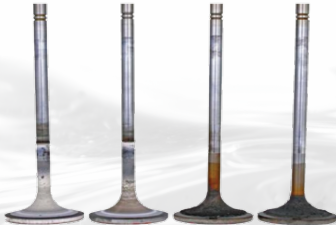
Exhaust Intake Valves show light deposits with no visible signs of recession.
