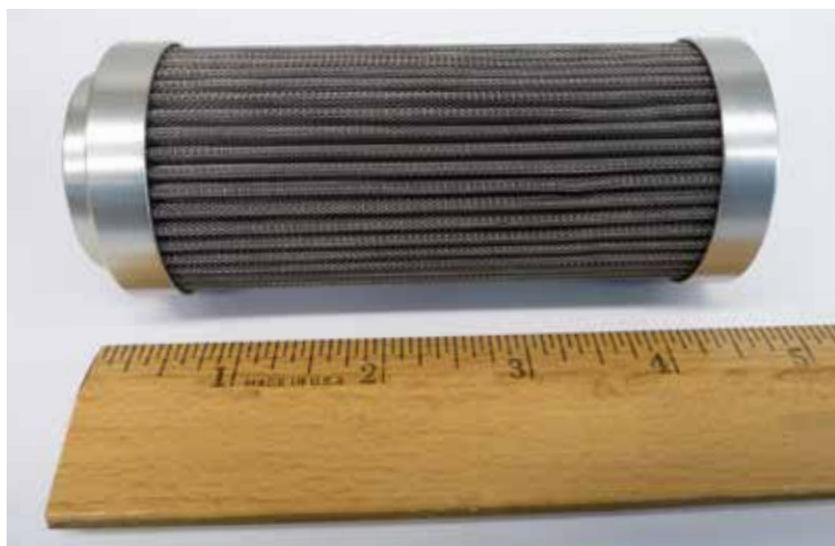
Clean Filter/Filter media from servo valve control system of GE 7 EA gas turbine at Chevron Sycamore Cogeneration Plant.
