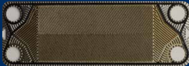
BEFORE CLEANING: Varnish film
